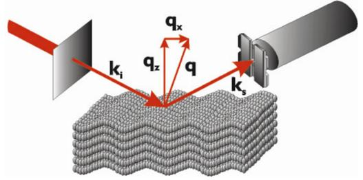
**Fig. 58:** Schematic scattering configuration for experiments on fluctuating smectic membranes.
